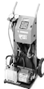
b.) ALL PURPOSE CHARGING STATION INCLUDES AUTOMATIC EVACUATION, OIL INJECTION, RECHARGING, ELECTRONIC CONTROLS TO ADJUST VACUUM PUMPING TIME AND LEAK DETECTION
